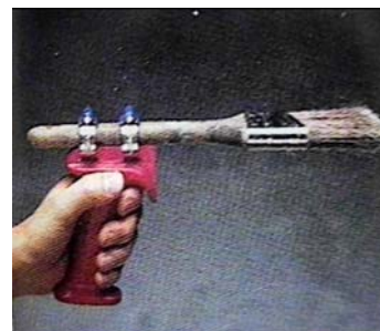
Pistol grip add-ons can also be used to keep the hand and wrist in neutral postures.
