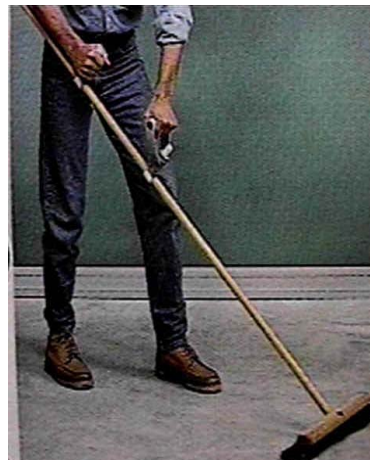
Pistol grip add-ons reduce bending and can be added to shovels, brooms, rakes, and other tools.
